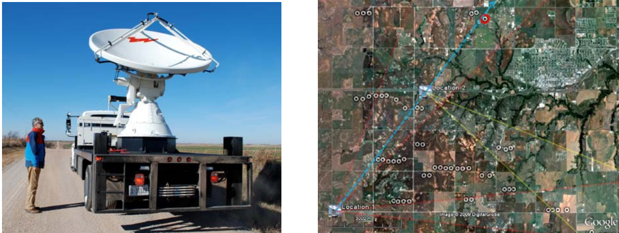
Figure 6: Picture of the NOXP mobile radar used in the polarimetric study (left). Also provided in the right panel is a map of the experimental region near Weatherford, OK. The white circles on the map represent the locations of the wind turbines. The two radar locations are marked with a picture of the radar along with coverage angles marked with red lines (Location 1) and yellow lines (Location 2). The
