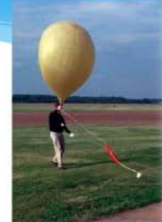
Launching a radiosonde
