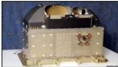
Advanced Technology Microwave Sounder (ATMS)
