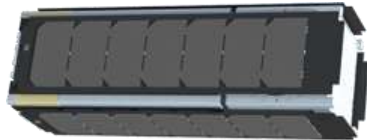
Bus with solar panels in launch position 10 cm × 10 cm × 34 cm
