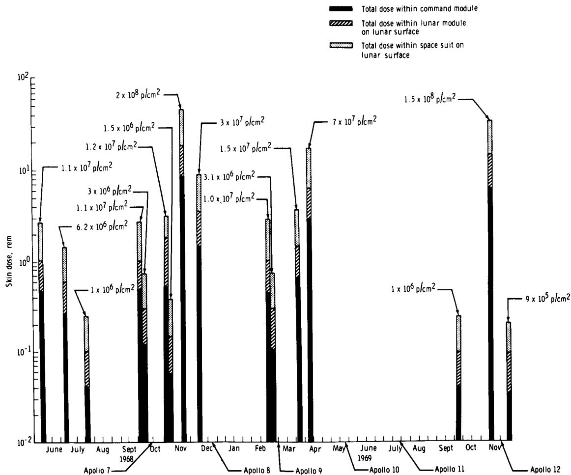
Figure 1. - Radiation-dose estimates for particle events between June 1968 and December 1969.
