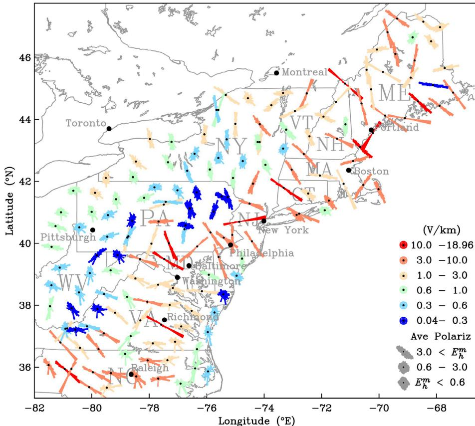
Map showing maximum geoelectric field, as a function of azimuthal direction (declination), realized at sites across the NE United States from 1983-2016.
