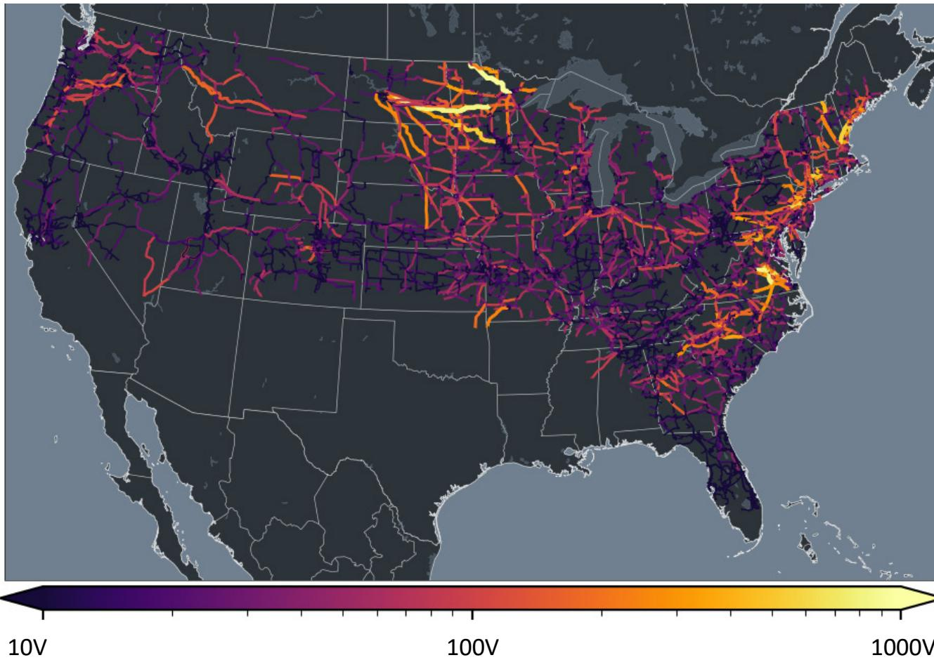
Obtained by integrating geoelectric fields along power lines.
