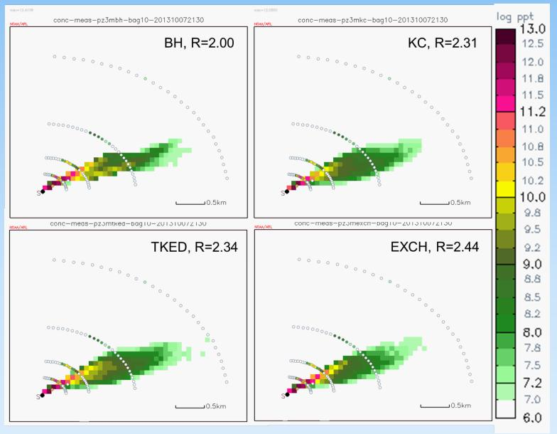
The larger horizontal velocity variance in the EXCH-obs generated a wider plume than the one in the EXCH simulation.
