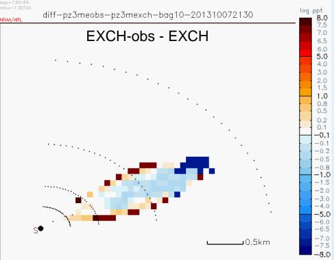
The TKED plume moved further away from the source location than EXCH plume. Near the source (200 and 400 arcs), EXCH had higher concentrations than TKED.
