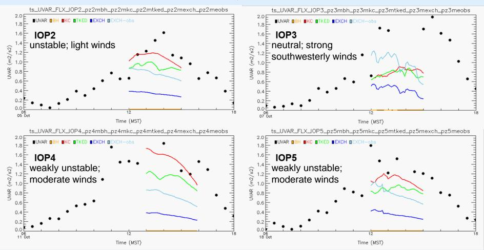
The scaling factor used in the BH mixing was too small causing significant underestimation of the u-variance. KC and TKED mixing had reasonable u-variances with a small underestimation.
