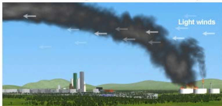
Plume Rise in Light Winds with Neutral Stability
