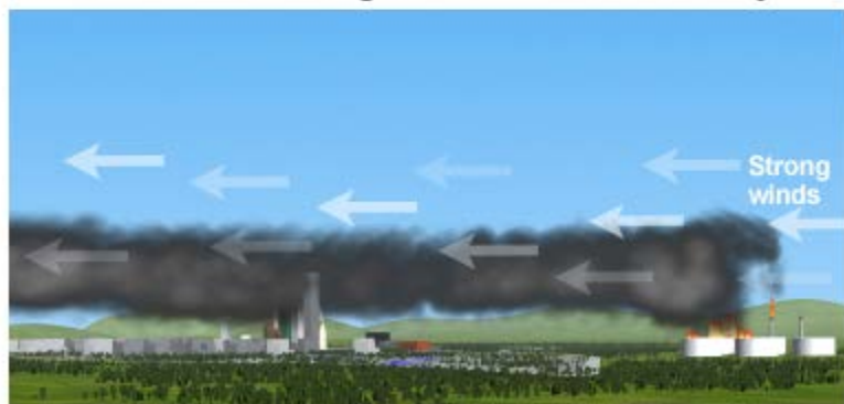
Plume Rise in Strong Winds with Neutral Stability
