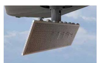
New Multi-mode radar replaced old Lower Fuselage system after 2017 hurricane season Weather mode with turbulence detection and Doppler spectral profile within 40 nmi Strip-SAR mode for surface roughness and scatterometry Spot-SAR, AIS, and Air-to-Air for tracking vessels and aircraft
