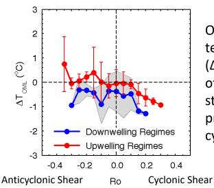
Ocean Mixed Layer (OML) temperature response  $(\Delta T_{OML})$ , based on 79 pairs of collocated pre- and instorm ABXT temperature profiles from eight tropical cyclones.
