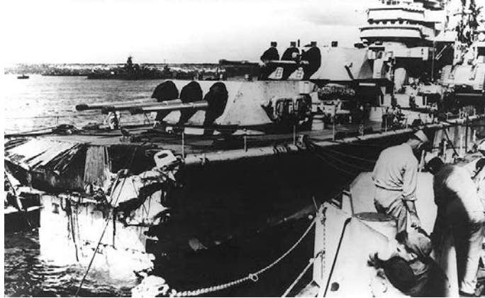
Photo # NH 98249 USS Pittsburgh at Guam after losing her bow in a typhoon
