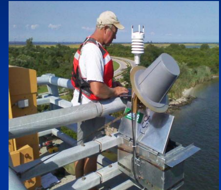
RDG installed on bridge over State Boat Channel at Captree Island, NY for Hurricane Irene.
