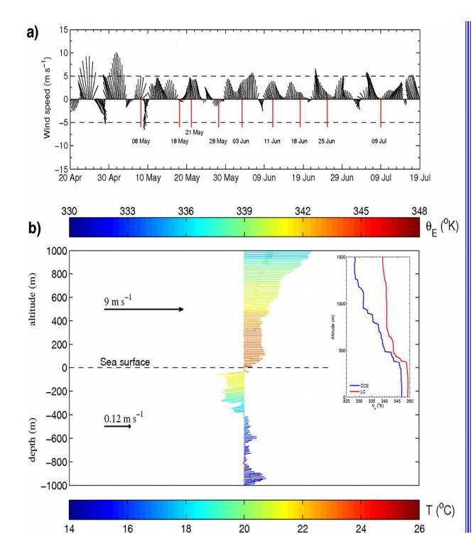
Upper: adjusted surface winds (10-m) at NOAA Data Buoy 42040 located ~55 km NE of DWH-Red lines depict day of the flights.
