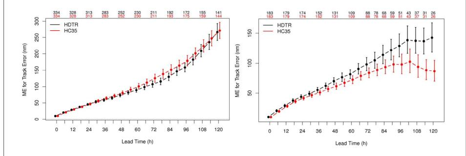
Experimental configuration improves track for AL but degrades for EP
