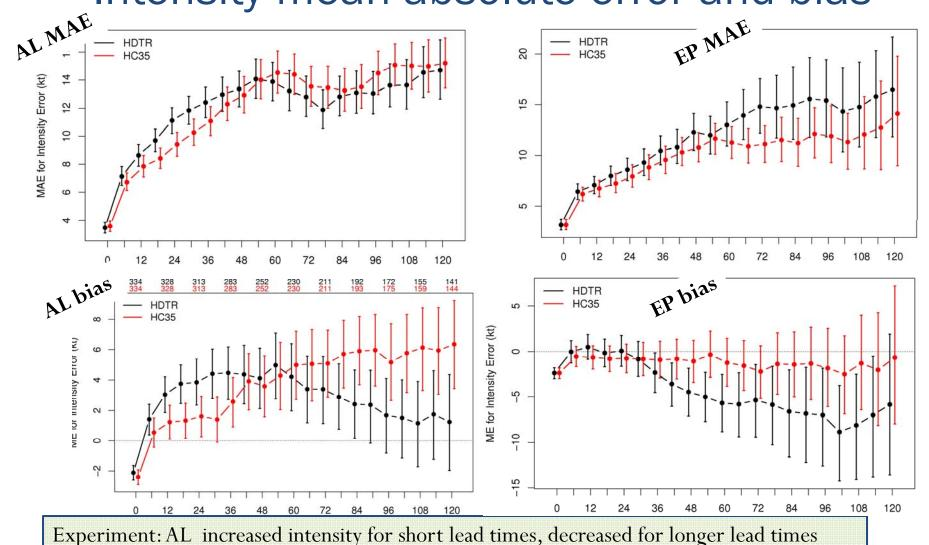
Experiment: AL increased intensity for short lead times, decreased for longer lead times EP decreased (degraded) intensity
