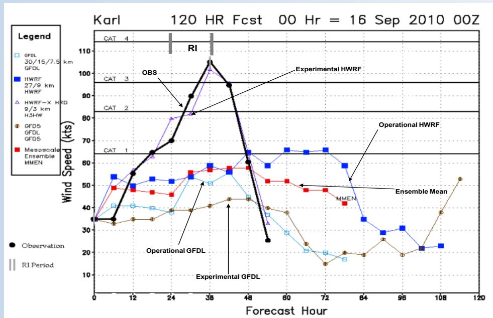
Wind speed forecasts from various models. The observed wind is shown as the black line. MME is the mean of HWRF, GFDL, and Experimental HWRF (Gopalakrishnan - personal comm.).
